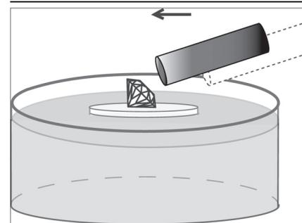
Fig. 6. Gem placed on buoyant material with largest flat face exposed for best interaction. Magnet is slowly moved toward gem and behaviour is observed. Good for observing subtle responses.
